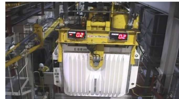
The final flask of fuel in Wylfa's fuel handling area (image: NDA)
